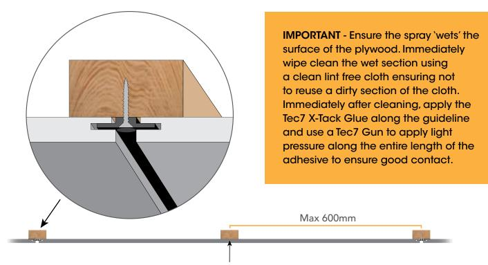
Fasten with Tec7 X-Tack Glue. Both surfaces must be cleaned first with Tec7 Multiclean Foam Spray.
